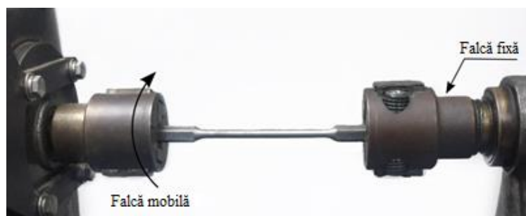
Fig. 2.26. Mașină de teste la torsiune. Reprinted with permission from ([17] S.A. TORO, P.M. ARANDA, C.M. GARCÍA-HERRERA, D.J. CELENTANO, ANALYSIS OF THE ELASTOPLASTIC RESPONSE IN THE TORSION TEST APPLIED TO A CYLINDRICAL SAMPLE, MATERIALS. 12 (2019) 3200). Copyright (2019) The Author(s).
